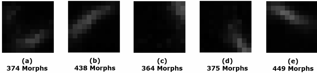
Fig. 7. Resultant receptive feature maps after 2000 training iterations on the image in Fig. 5, without using the sensory-invariant driver. Focus points were selected randomly each iteration. Orientation-selectivity is apparent in fields (b) and (e), but not in the other fields.
