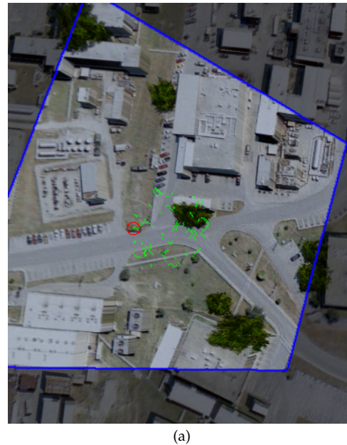
Fig. 5. Search image registered to survey view. Using the found homography, the search image is registered to the survey view. Green trails indicate the paths taken using the histogram shift procedure from each seed point, and the final result of the search is shown by the red circle.
