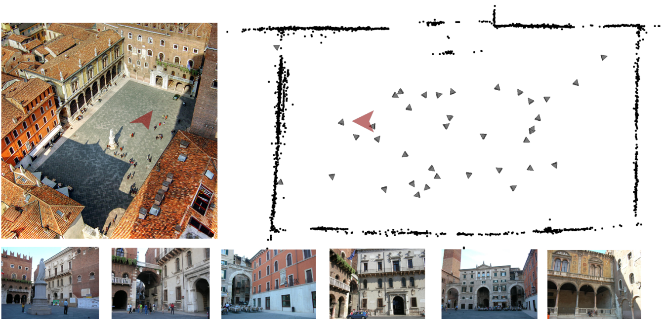
Figure 7. Autocalibrated reconstruction from a collection of photos (taken by the same camera) of the Piazza dei Signori in Verona, Italy. The reconstruction is shown from a top down orthographic perspective. The reconstruction consists of 39 views and a total of 2971 structure points. Some images from representative views are shown along the bottom (the aerial view was not used in the reconstruction and is presented only for reference).
