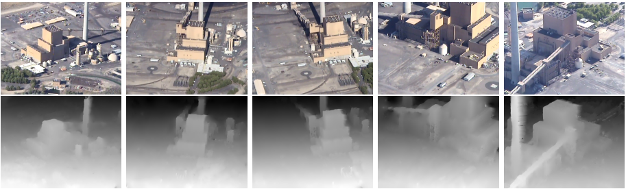
Fig. 3. Selected keyframes and associated inverse depth maps estimated by TGV-SLAM on the Boardman dataset.
